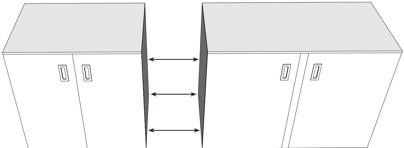
Drill holes in the prepared places - drill bit 5 mm
